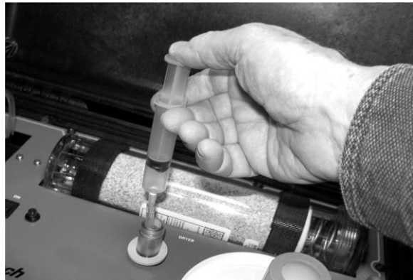
Figure 8-2. Filling the Saturator
