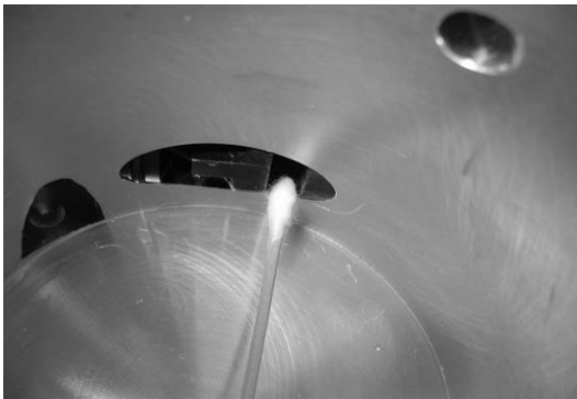
Figure 14-1. Cleaning mirror with swab
