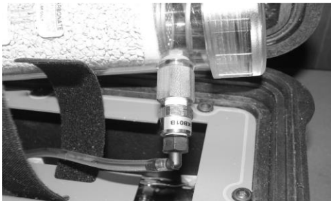
Figure 14-2c. Disconnect clear tubing
