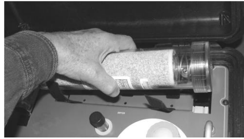
Figure 14-2b. Lift out the Dryer
