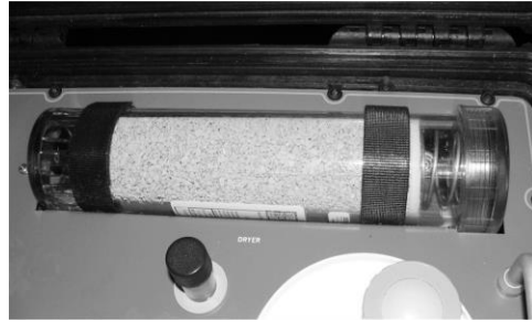
Figure 14-2d. Replace the Dryer
