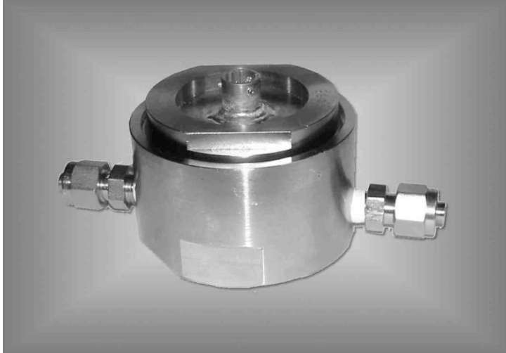
Figure 3-1 The Phosphorous Pentoxide ( P_2O_5 ) Moisture Sensor
