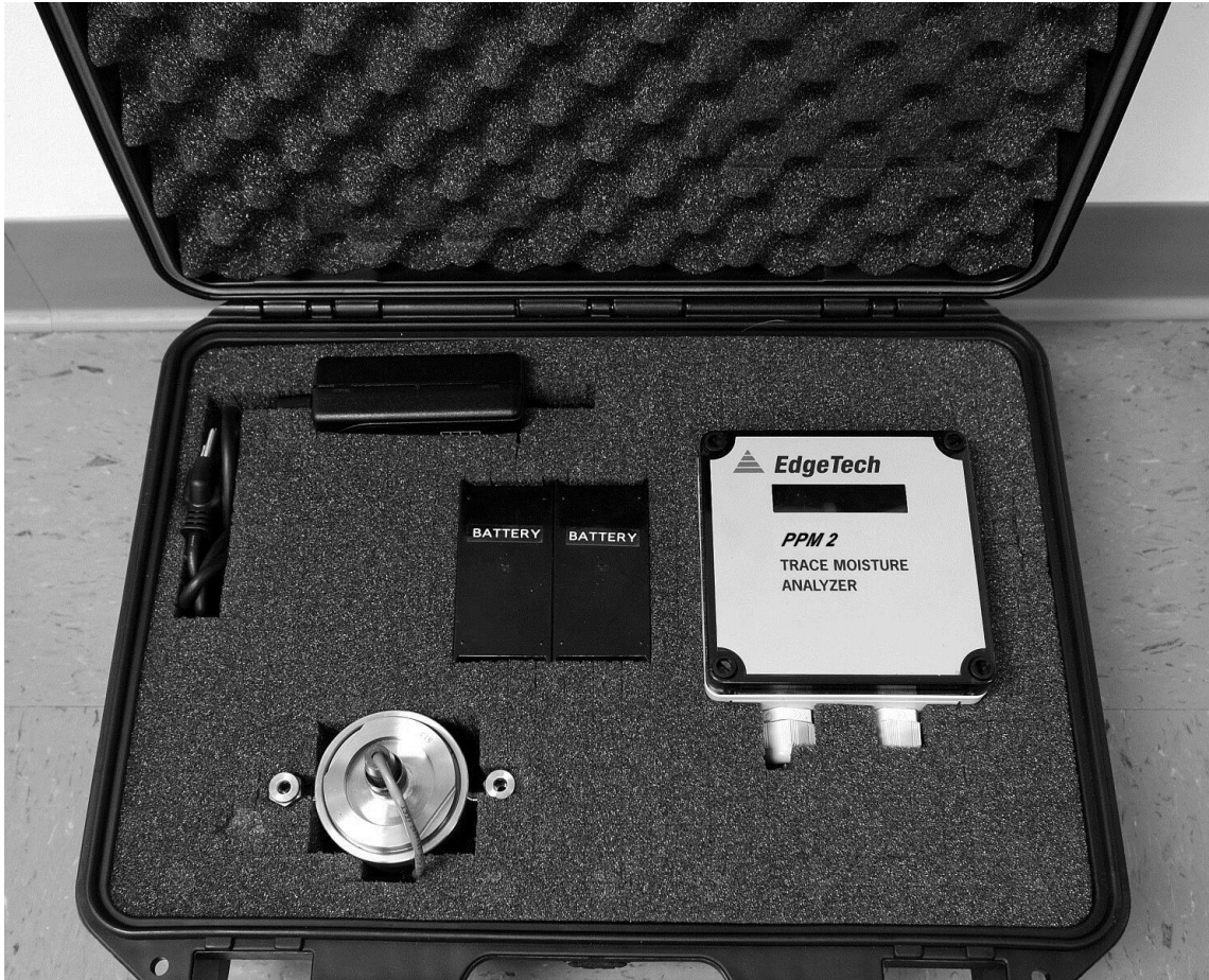
Figure 3-3 The PPM2 Portable Trace Moisture Analyzer
