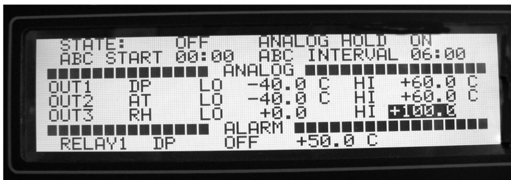
Figure 12-3. Setting the Analog Output 3 (RH) Range
