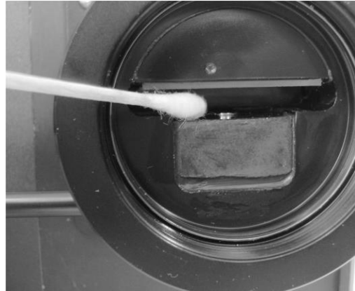
Figure 14-1. Cleaning the Mirror
