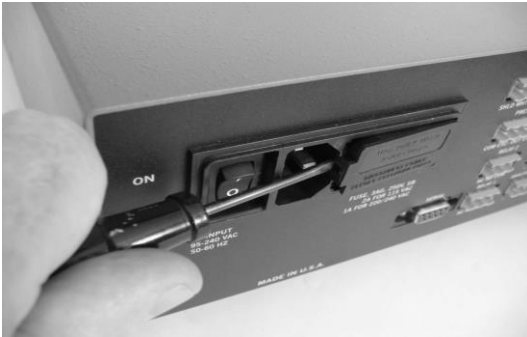
Figure 14-2a. Opening the Cover
