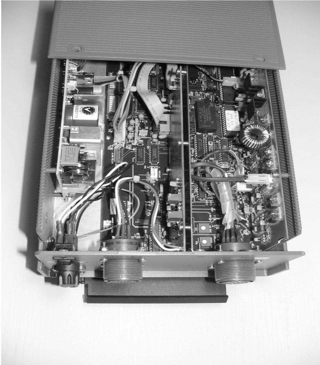
Figure 5-4 View of Interior with Top Cover Removed
