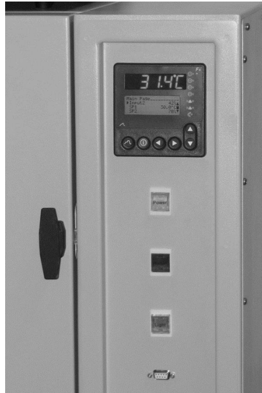
Figure 5-3 Controller and Pilot Lights
