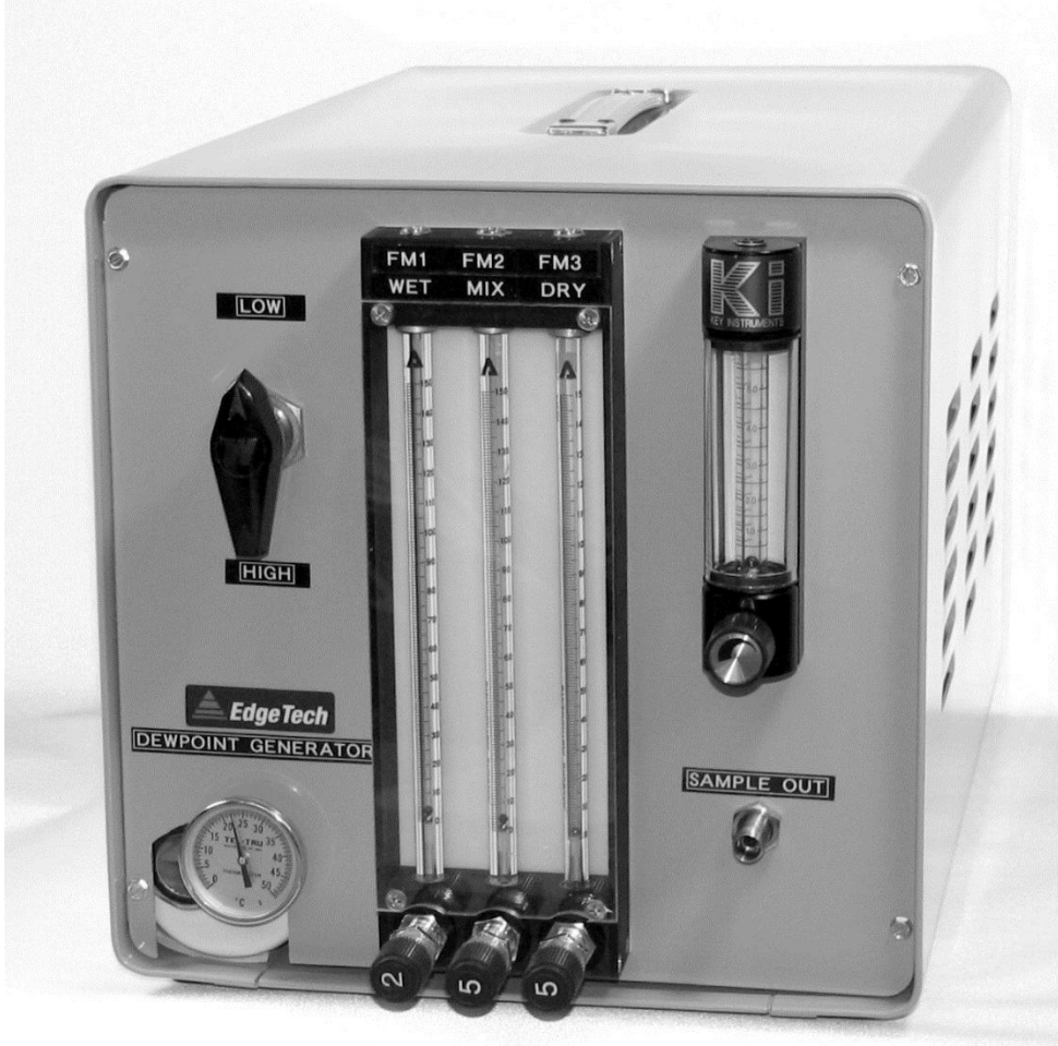
Figure 6-1 DewGen Dew Point Generator
