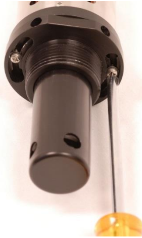
Fig 7. The collar is removed by first loosening the two set screws and rotating the collar until the heads of the set screws can be slipped through the collar slots. Keep the O ring in site as it needs to be repositioned after cleaning and reassembly of the NPT collar.
