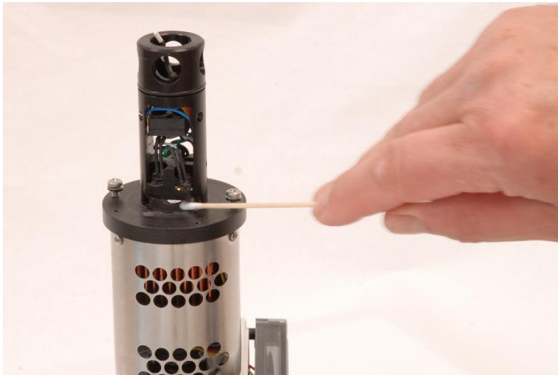
Figure 10. Mirror is exposed for cleaning with a clean swab.
